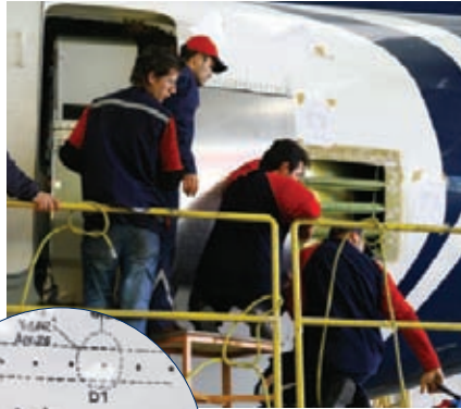
This 737 arrived at myTECHNIC with a large number of dents around the rear door caused by ground support equipment. As this was outside Boeing's repair limits, the Turkish company developed its own repair scheme that was approved by the OEM (photo: Ian Harbison)
